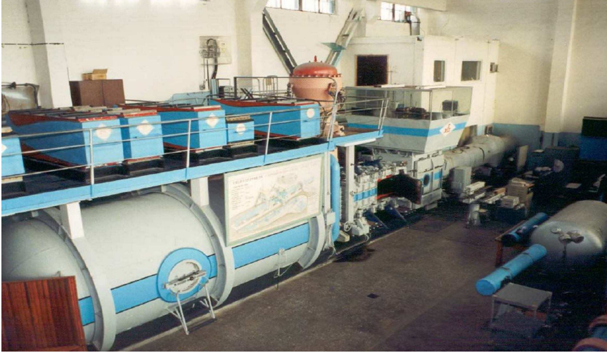
Figure 4.1: Photograph of the blow down wind tunnel T-313.
