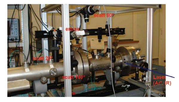
Fig. II.2.6: Picture of the scattering/extinction set-up employed on the big shock tube.
