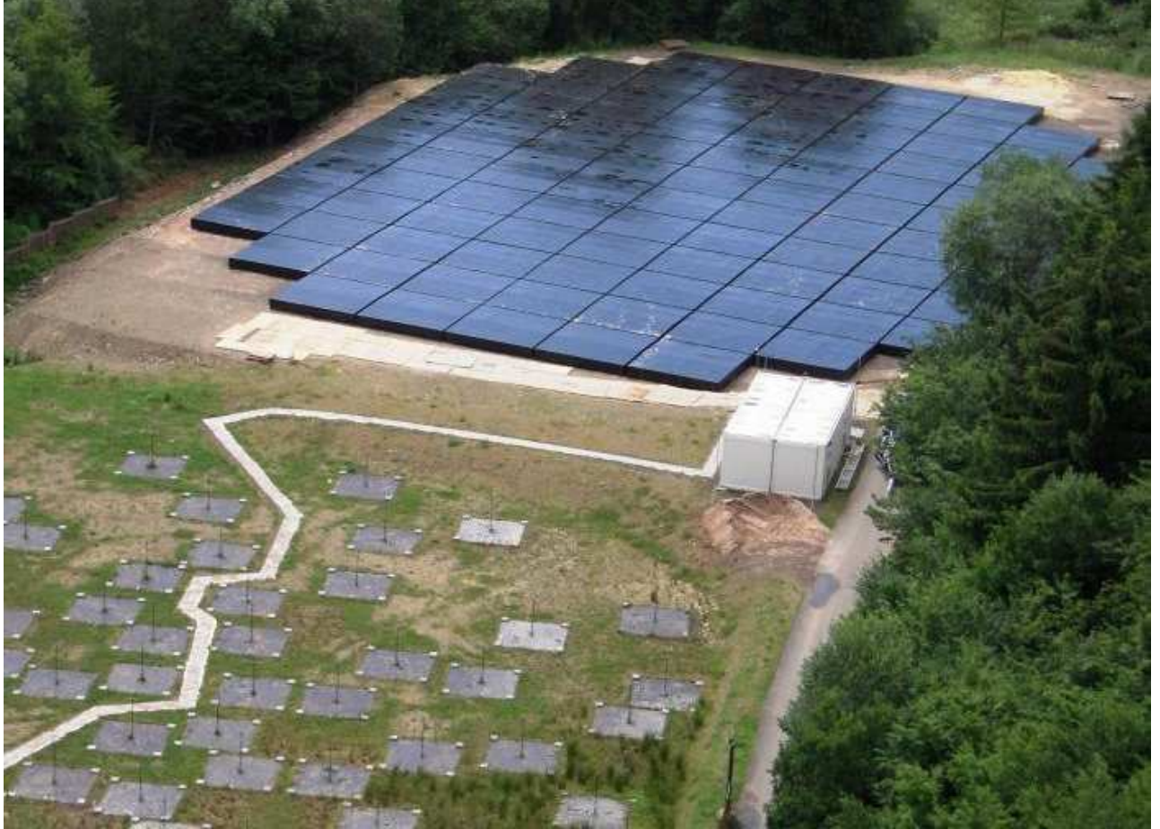
Figure A.1: LOFAR station at the Effelsberg site (Germany). Bottom left : the low frequency array (30 MHz- 80MHz). Top the high frequency array (110 - 240 MHz). Each black box is itself an array of high frequency antennas. Copyright of the Max Planck Institute for radio astronomy, ASTRON and LOFAR.
