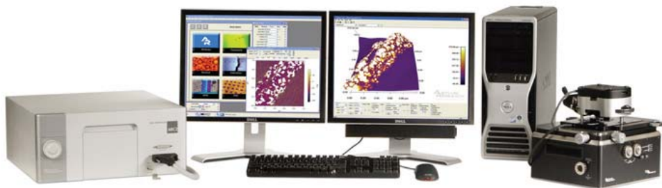
FIGURE 38 – Microscope à force atomique de type MFP3D – BIO TM Asylum Research Santa Barbara, CA .
