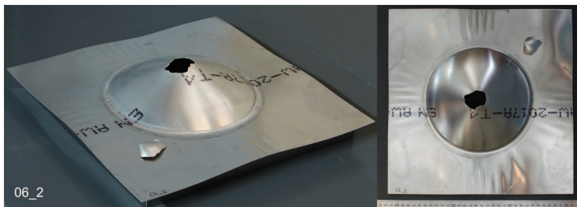
Fig. A2-11. Tested plate 06_2 (0.6 bar)
