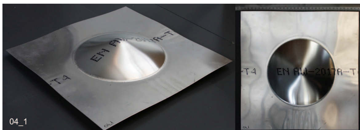
Fig. A2-5. Tested plate 04_1 (0.4 bar)
