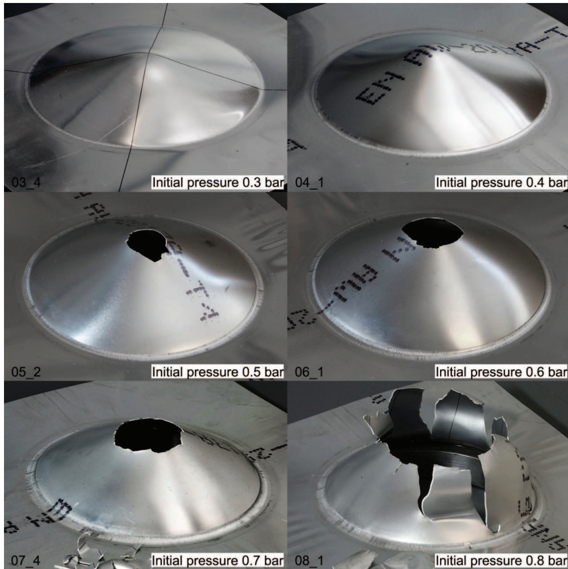
Fig. 4-12. Plates after experiments
