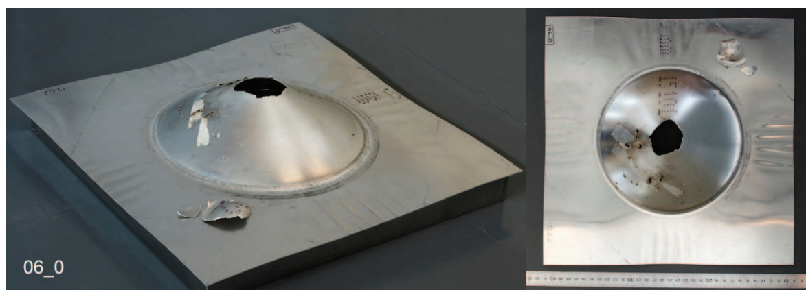
Fig. A2-9. Tested plate 06_0 (0.6 bar)
