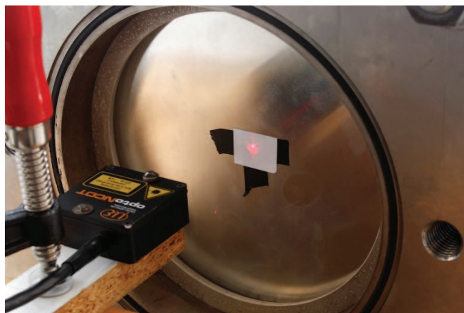
Fig. 4-15. Optic sensor measuring deflection of the plate
