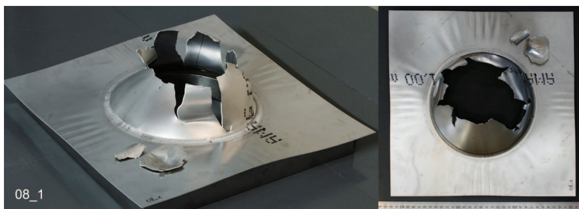
Fig. A2-17. Tested plate 08_1 (0.8 bar)
