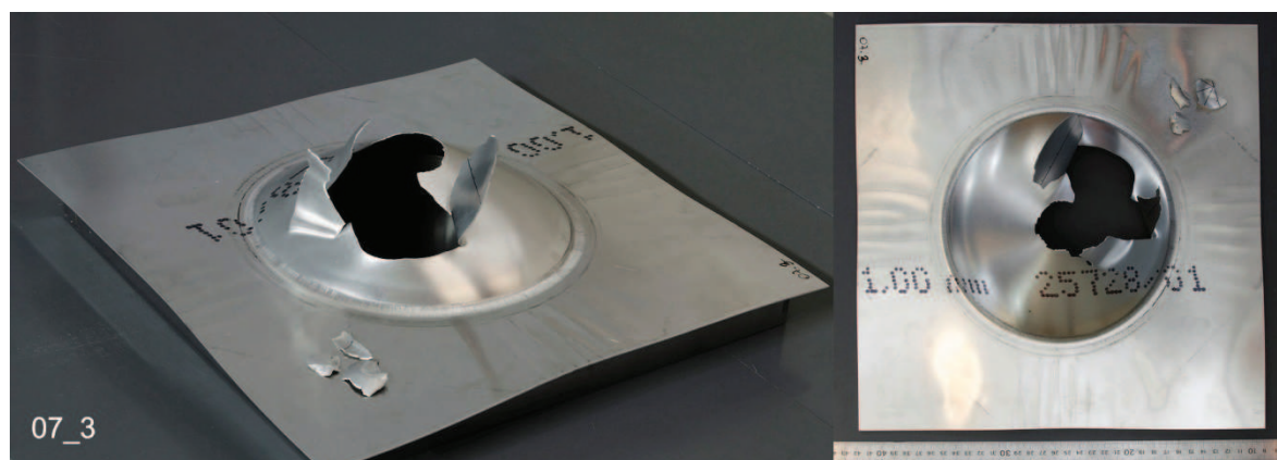
Fig. A2-15. Tested plate 07_3 (0.7 bar)
