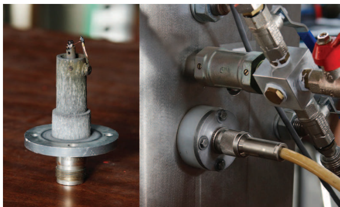
Fig. 4-6. Igniter and its installation
