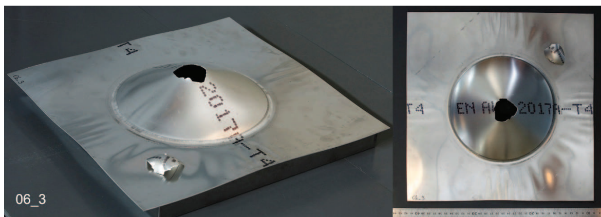
Fig. A2-12. Tested plate 06_3 (0.6 bar)
