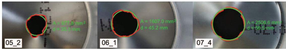
Fig. 4-17. Equivalent hole diameter measurement
