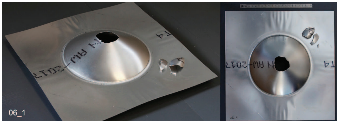
Fig. A2-10. Tested plate 06_1 (0.6 bar)
