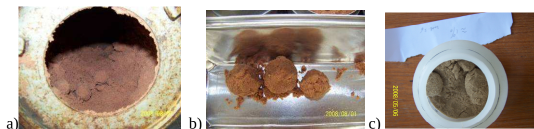
Figure 5-21 a) Wet sand stuck to the wall of tumbler even during rotating. b) Some “sand balls” were produced after tumbler rotating. c) At water content 1%, some aggregate was created.
