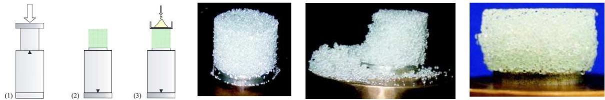
Fig. 4-14 LEFT Experimental device (see description in Soulié et al. 2006), First picture the cylinder of wet glass bead before mechanical testing; two last pictures: glass bead cylinders at 1 and 10% water content respectively, at the end of the test: brittle and ductile failure respectively. For brittle material, failure is caused by the break down of the bonds and propagates subsequently into the material (the tensile strength is not controlled by the average stress but by the largest local stress). For ductile material, the shear strengths controlled by the mean tensile force (Soulie et al., 2006).
