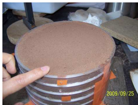
Figure 5-33 There can be some holes in the border, need to be filled carefully with finger. Otherwise, the white marker (glass beads) can leach from these holes.
