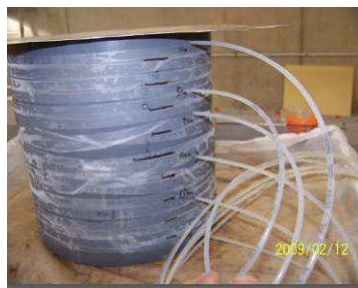
Figure 5-28 Micro-tensiometers were inserted in different layers (1, 5, 9, 13, 17 cm counted from the bottom).
