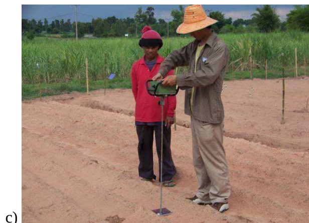
Figure 5-15 Mechanical characteristics measurement. a) measuring shear strength by scissometer, b) measuring resistance to penetration by pocket penetrometer, c) measuring resistance to penetration by datalogger penetrometer.
