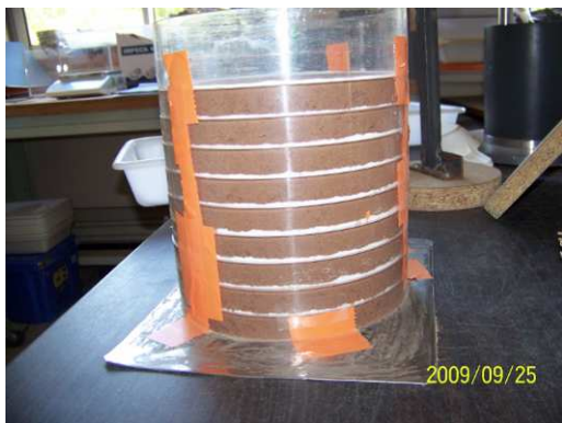
Figure 5-36 A final prepared cylinder, with marker in every two centimeter layer.
