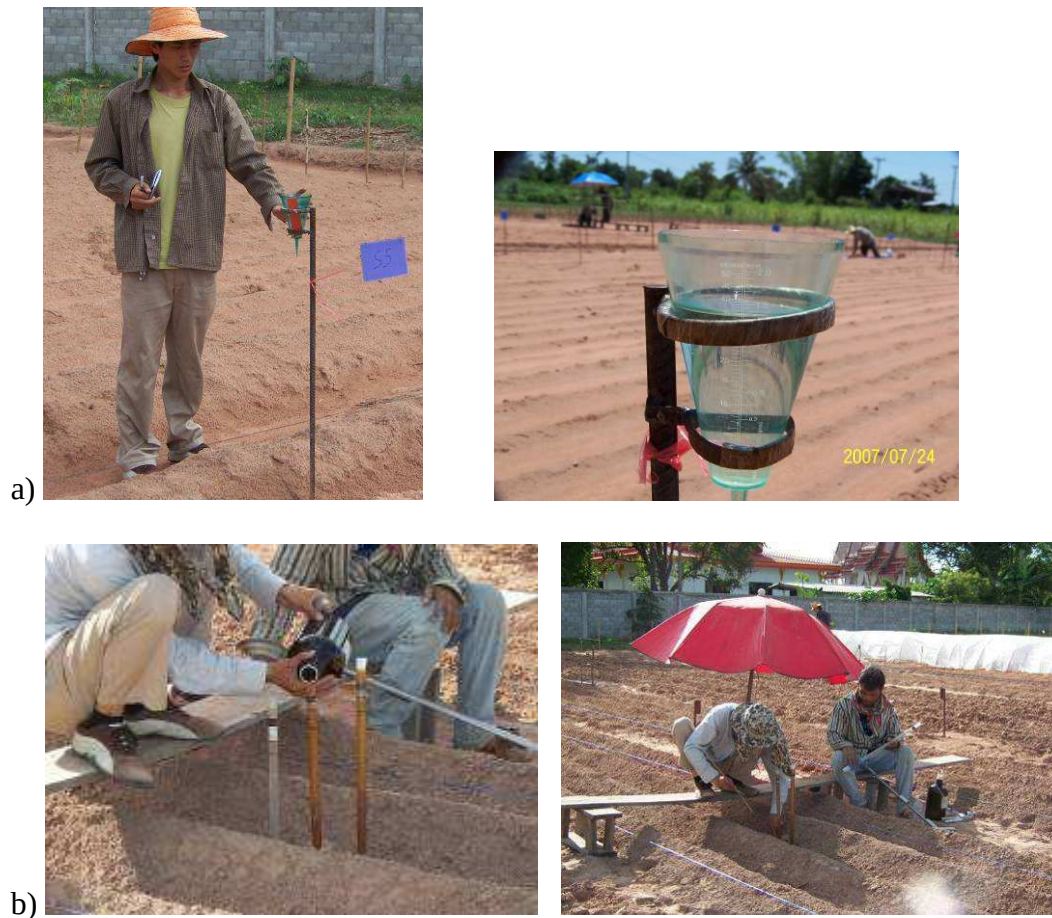
Figure 5-13 a) Rain gauge was installed in the field to measure rainfall. b) tensiometers were installed to measure soil water potential. Notice when we were working, a “wood bridge” was used to prevent disturbing the soil.
