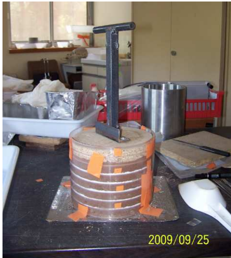
Figure 5-31 Push by a plate until the certain height.
