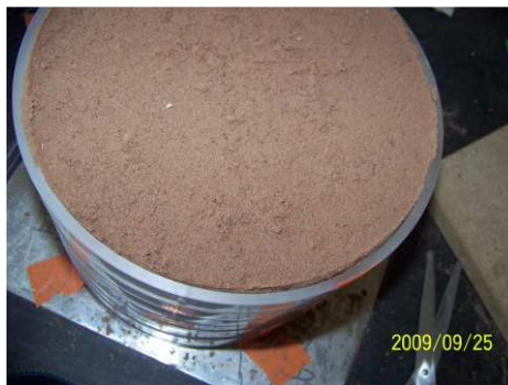
Figure 5-33 There can be some holes in the border, need to be filled carefully with finger. Otherwise, the white marker (glass beads) can leach from these holes.
