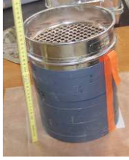
Figure 5-25 A 2 cm-hole sieve was used to let the wet sand pass by. It produced a loose structure.
