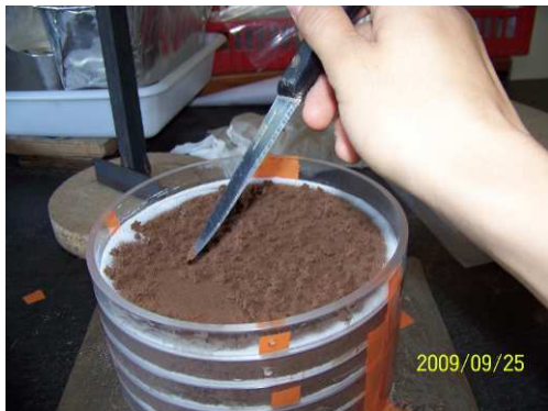
Figure 5-35 Between each two layers, the soil surface was reploughed a little bit, in order to increase the water flow, and prevent the “border effect” (water accumulate in the surface).
