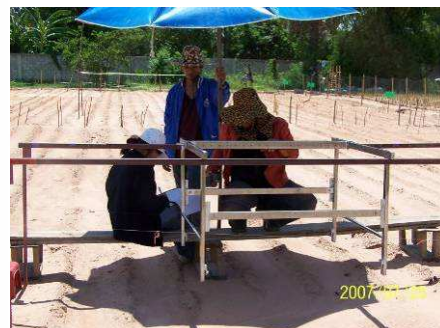
Figure 5-10 Set up for Exp.1 to measure the surface topography and soil height of a 1 m 2 plot.
