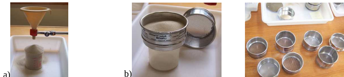
Figure 5-18 Different ways to fill the columns: a) point source deposit with funnel, b) rain deposit with sieve, different sizes of sieves were used.
