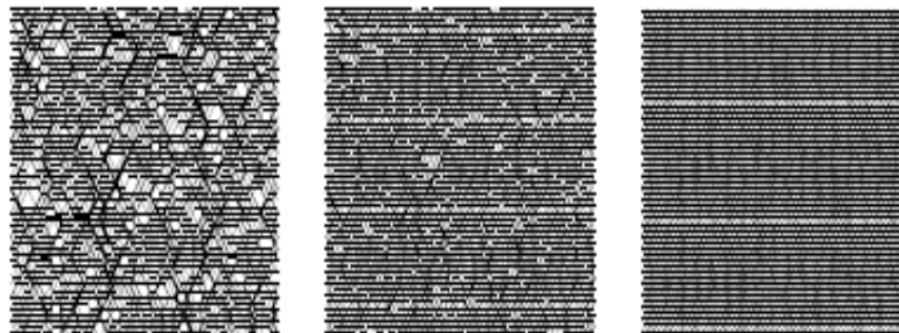
Fig. 3-12 The contact are perfectly rigid at the left side and become softer for center and right figure: with softer contacts, the distribution becomes more homogeneous (Atman et al., 2005a; Atman et al., 2005b).
