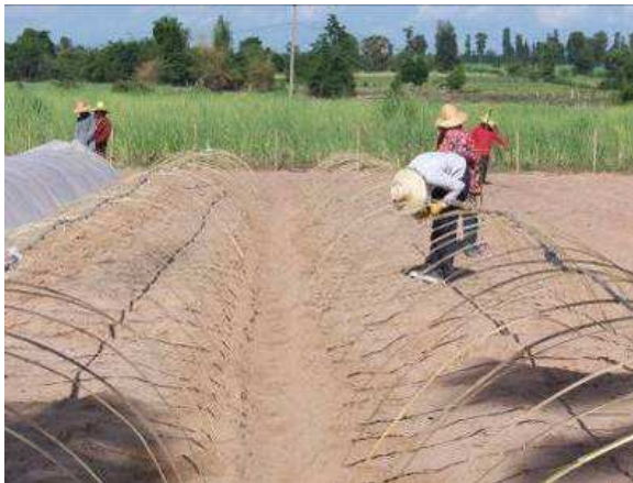
Figure 5-7 In Exp.2, plastic sheet were used to protect the soil from rainfall, therefore, a dry (Y) initial water content was obtained when ploughing.
