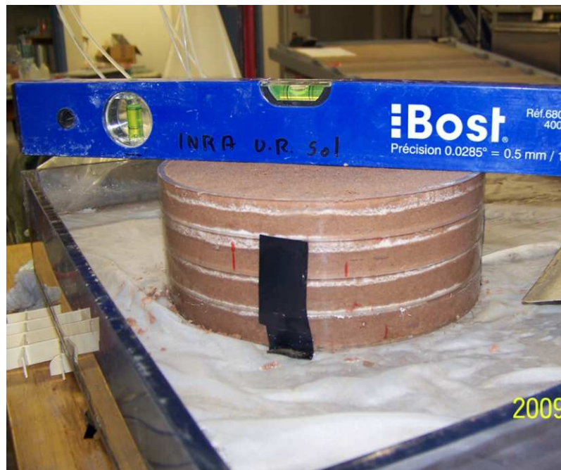
Figure 5-29 When cutting, a “spirit level” horizontal ruler was used to check if the cutting is flat.
