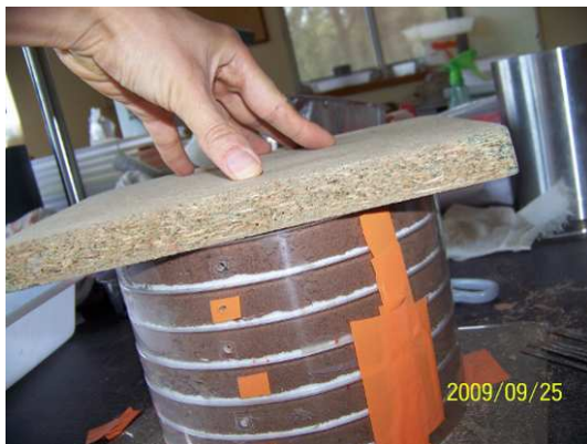
Figure 5-32 Use a plat to plush, make the surface flat.
