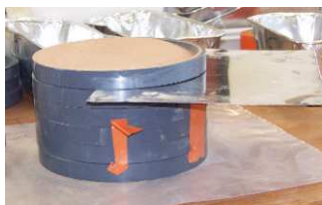
Figure 5-23 Cylinders were connected by adhesive tape. An iron plate was used to penetrate each layers.
