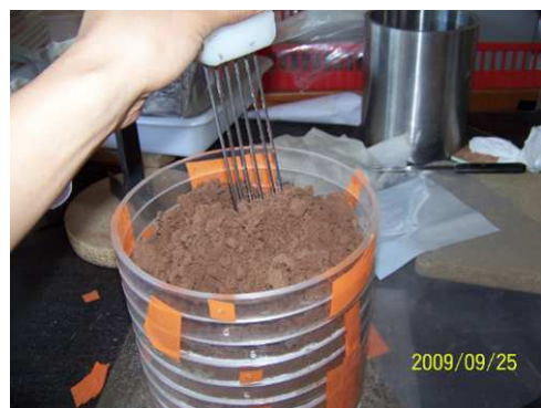
Figure 5-30 Fill a certain amount of soil in each 2 or 4 cm cylinder.
