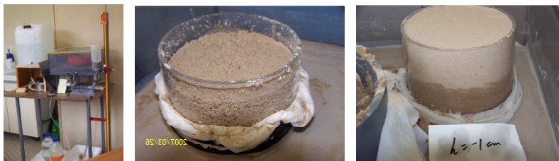
Figure 5-22 Wet sand column affected by capillary force. a) water suction table, b) wet sand after 2 days in suction table with h=0 , c) dry sand can not be totally wetted by capillary force at h= -1 hPa.
