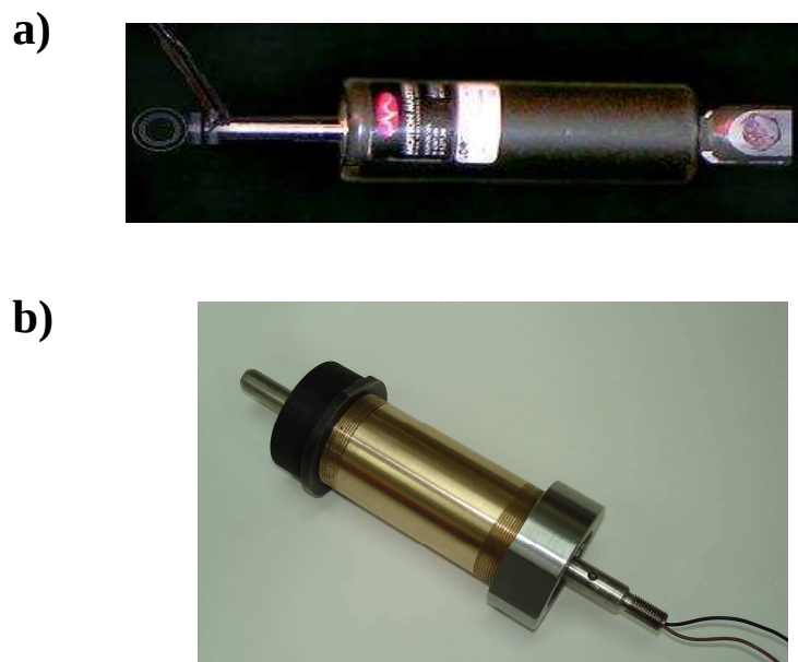
Fig. 2.2. View of research objects: (a) LORD RD 1005 – 3 shock absorber; (b) T-MR SiMR 132 DG damper
