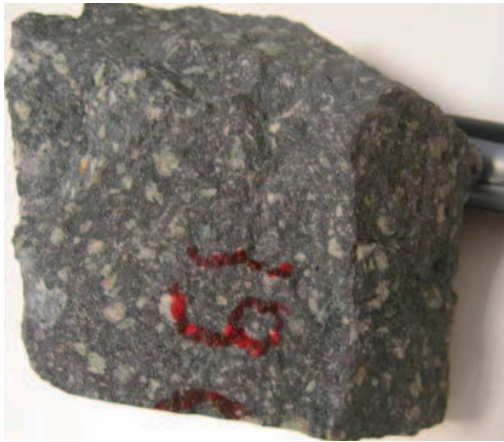
Fig. 3-12: Photographs of basalt from Yamansu magnetite deposit. (A) Hand specimen of basalt. Plagioclase phenocrysts are in white. (B) and (C) Photographs of basalt in plane-polarized light and reflected light from the same thin section, respectively. In the (B), the plagioclase shows multiple twins. In the (C), disseminated magnetite and hematite are observed in the fine grain groundmass, around the plagioclase phenocryst. (D) Photo showing relics of basalt in the massive garnet skarn. Relics of basalt are emphasized in dotted yellow lines; massive garnet skarn is in pale rose.
