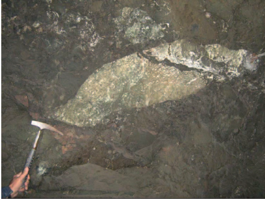
Fig. 3-13: Clasts of marble within altered basalt suggesting mafic magma stoping. The photo was taken in the gallery, about 200m underground. Potassium metasomatic alteration developed leading the formation of K-feldspar (in the pale red part).
