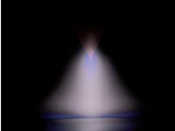
Figure 1. 5: Appearance of argon arc plasma [Tana-1].
