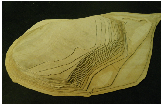
Figure 5.6.: Terraced model of the Bolund hill at 1/500 scale.
