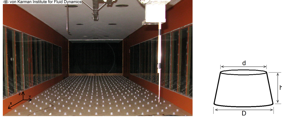
Figure 3.3.: Left: General view of the boundary layer generators: the grid, the fence (on the background) and the roughness elements. Right: Zoom on the cup dimensions (right)
