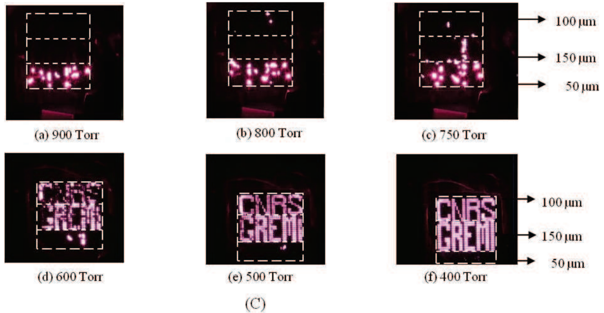
Figure 4.36: Effect of pressure variation in He gas environment on the arrays having different hole diameters 100, 150 and 50 \mu\text{m} on the same chip. (Dotted windows on the images indicate the border lines for different arrays)
