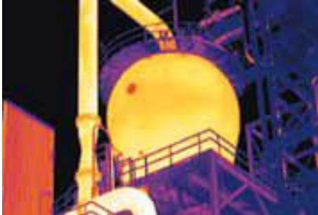
Figure 3.3: Thermal image of refractory insulation inspection on a petrochemical reactor [Flir, 2011]
