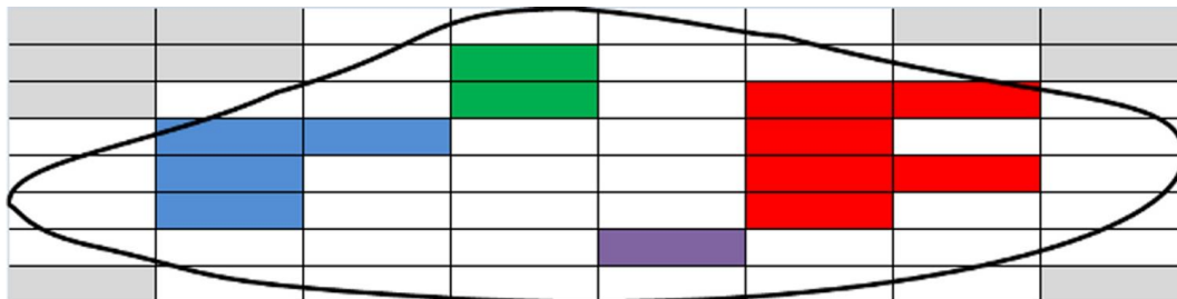
Figure 1: Simulation of the projection in a DRCS of a library having four clusters of occupied cells. The cells considered to be outside the DRCS are in gray, the DRCS contour is in black, the four clusters of occupied cells are colored differently.
