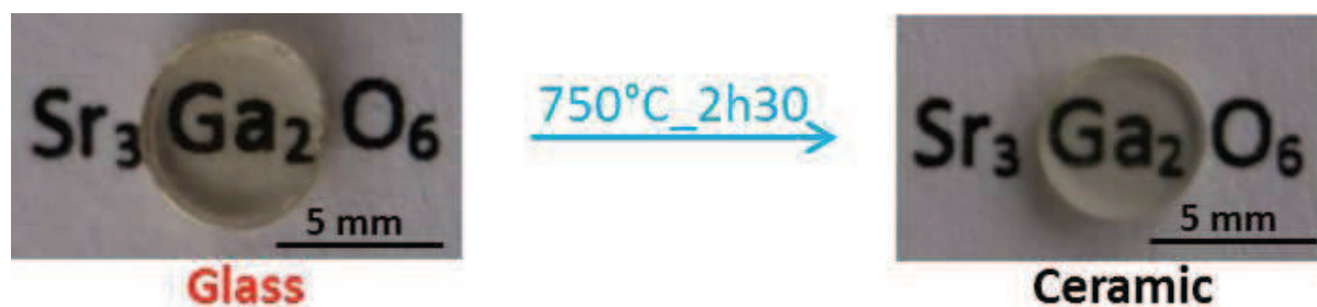
Figure 6 \text{Sr}_3\text{Ga}_2\text{O}_6 glass and the corresponding polycrystalline transparent ceramic obtained by thermal annealing of the glass at 750 °C for 2 hours 30 minutes
