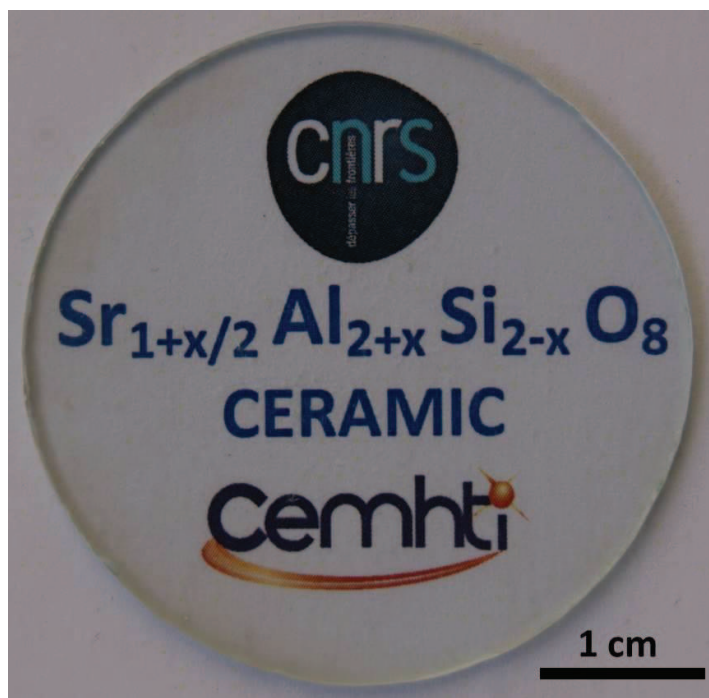
Figure 23 Photograph of the Sr_{1.1}Al_{2.2}Si_{1.8}O_8 ( x=0.2 ) transparent polycrystalline ceramic (1.5 mm thickness)
