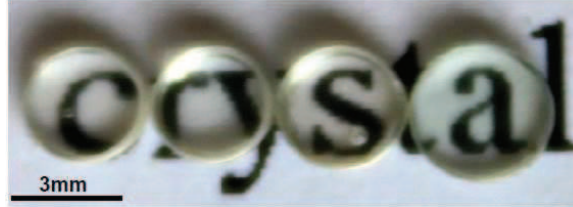
Figure 2 SrAl_2O_4 transparent single crystals elaborated by aerodynamic levitation coupled to laser heating system 31
