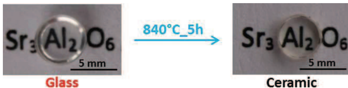
Figure 5 \text{Sr}_3\text{Al}_2\text{O}_6 glass and its corresponding transparent polycrystalline ceramic obtained by thermal annealing of the glass at 840°C for 5 hours
