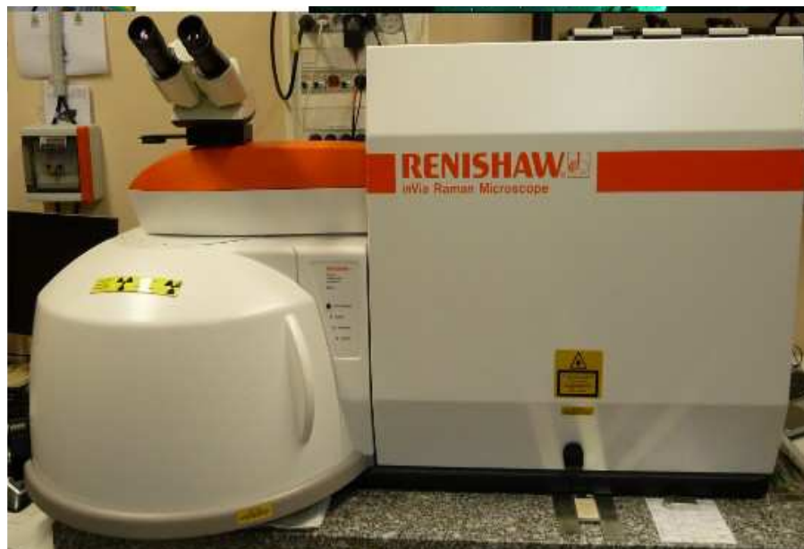
Figure 1.2. InVia Reflex Renishaw Raman system.
