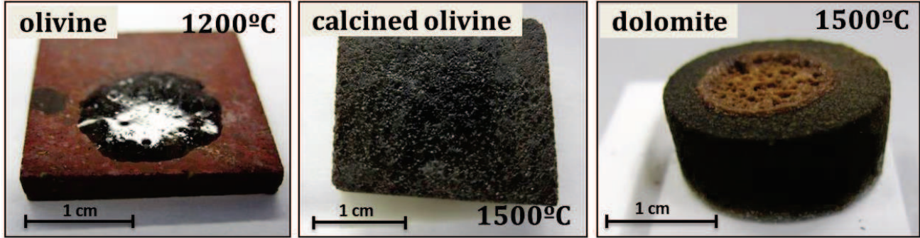
Figure IV-15: Olivine, calcined olivine and dolomite pastille after the wetting test
