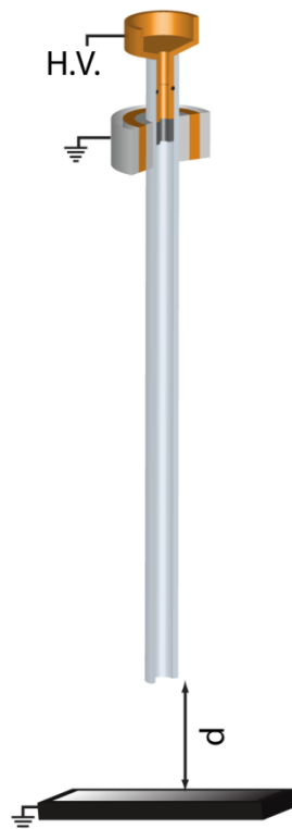
Figure 2.9: Setup of the PG with the target. d been the variable distance between the capillary outlet and the target.
