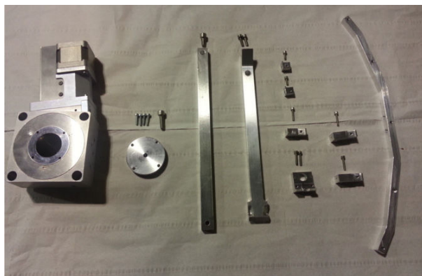
Figure 4.15: Parts that compose the rotating arm. From left to right: rotation stage, mechanical interface, horizontal and angled beams, beam/arch interface and probe holders, arch.
