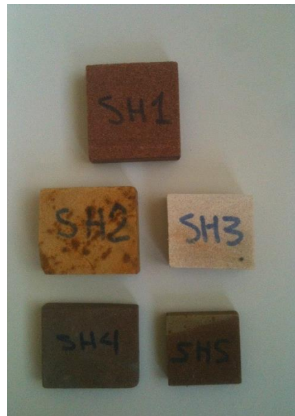
Figure 3-2 Adamswiller, Cleebourg and Rotbach sandstone rock samples
