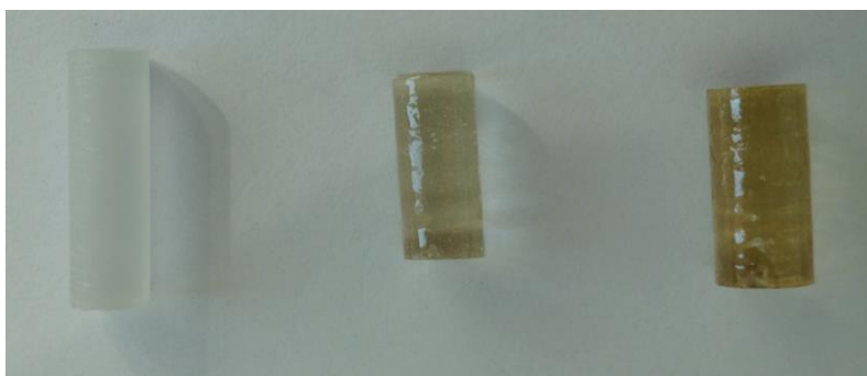
Figure II.1. Samples of BA60.10 ( left ) BA50.12 ( centre ) and BA42.14 ( right ) glasses illustrating increasing capacity of melts to incorporate Pt from the crucible.
