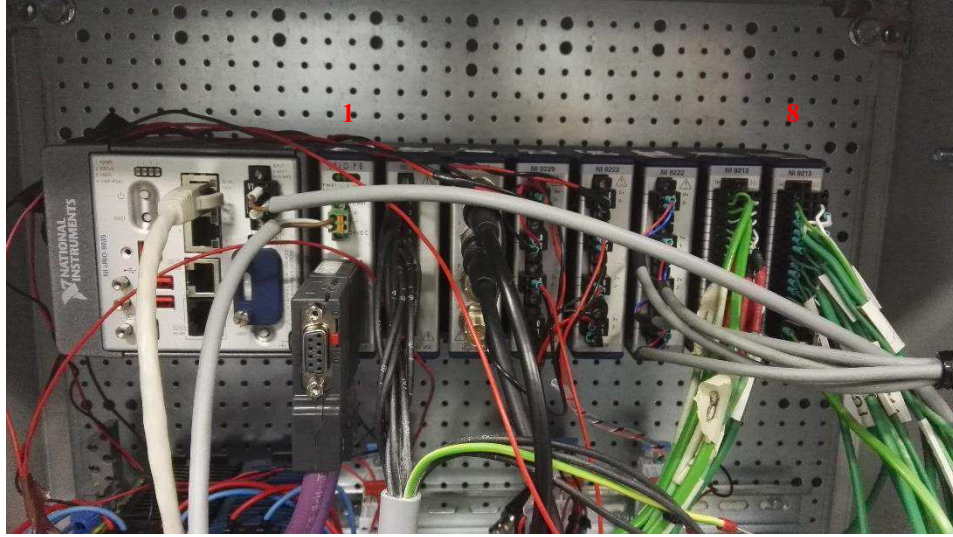
Figure 35: NI-9035 cRIO – final configuration
