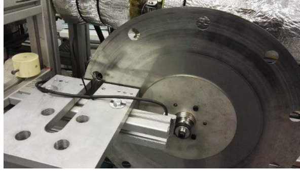
Figure 49: Thermocouple characterization apparatus – Rotating wheel
