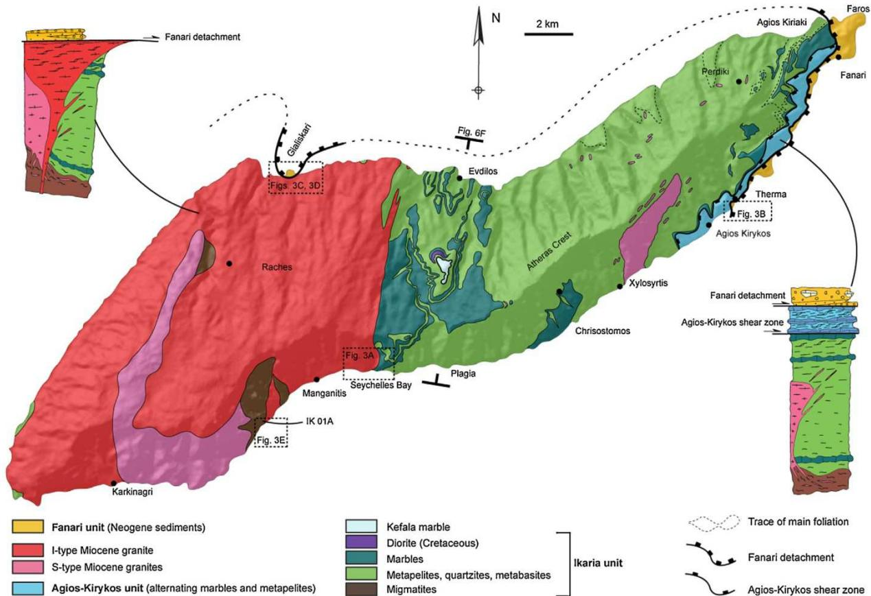
**Fig. 2.** Geological map of Ikaria. (a) New geological map of Ikaria proposed in this study. Lithologic outlines correspond to new field observations and a compilation of existing maps (e.g. Papanikolaou, 1978; Photiades, 2002b; Kumerics et al., 2005; Ring, 2007). Also indicated are two representative tectonometamorphic piles for the eastern and the western parts of Ikaria.
