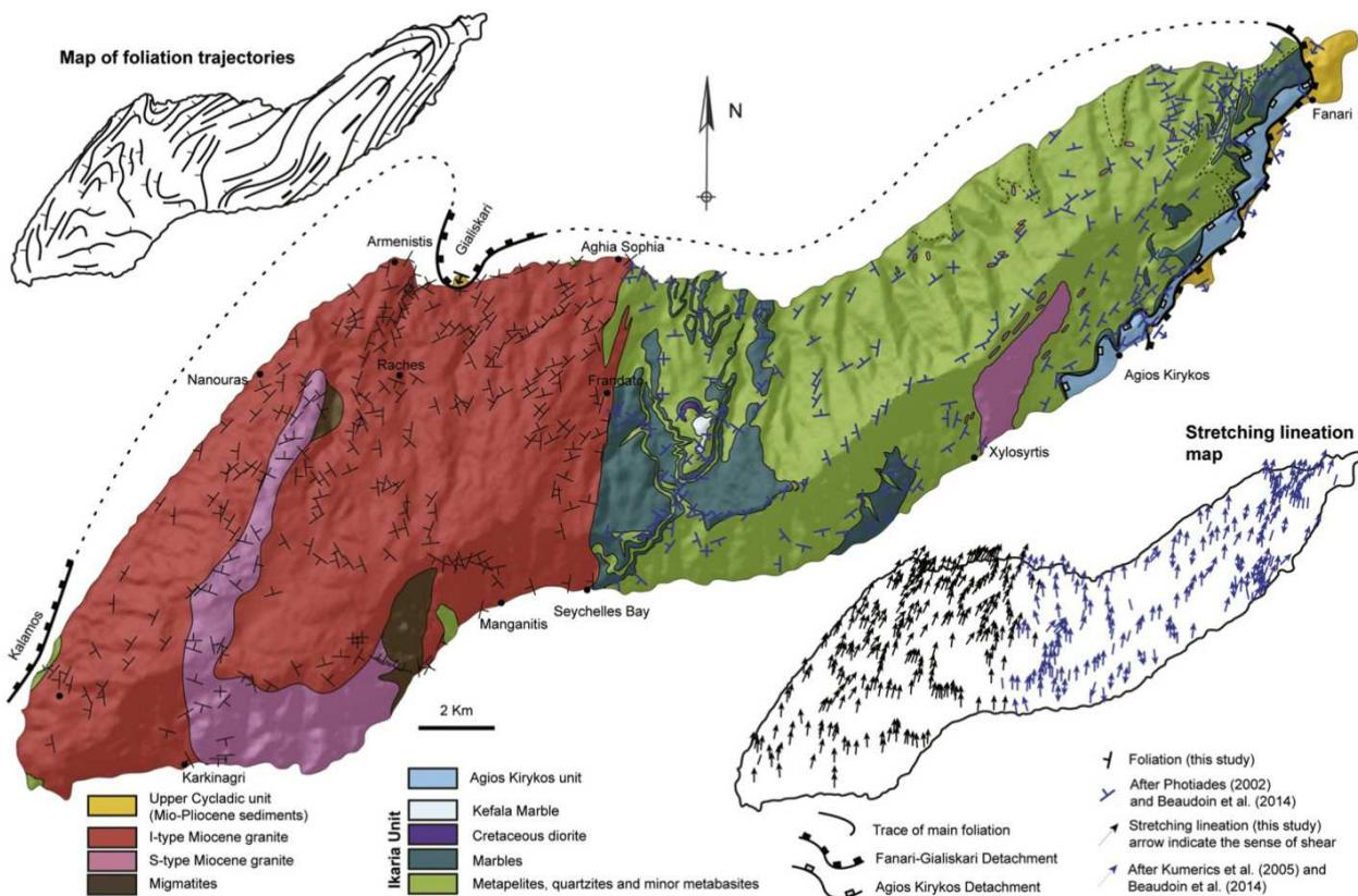
**Fig. 2.** New geological map of Ikaria Island showing the tectonic units, the two Gialiskari and Agios Kirykos detachments, foliation trajectories, stretching lineation measurements and localities cited in the text.
