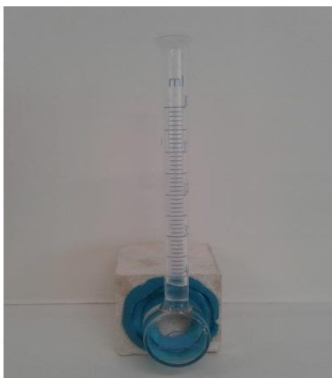
Figure II-28 Tube de Karsten
