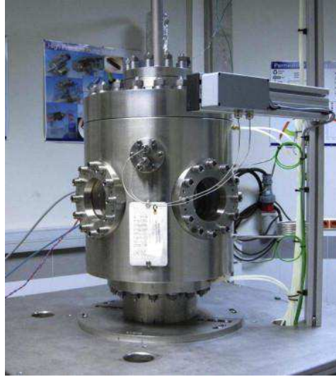
Figure 24 Constant-Pressure Flow (CPF) chamber of CMT [110].
