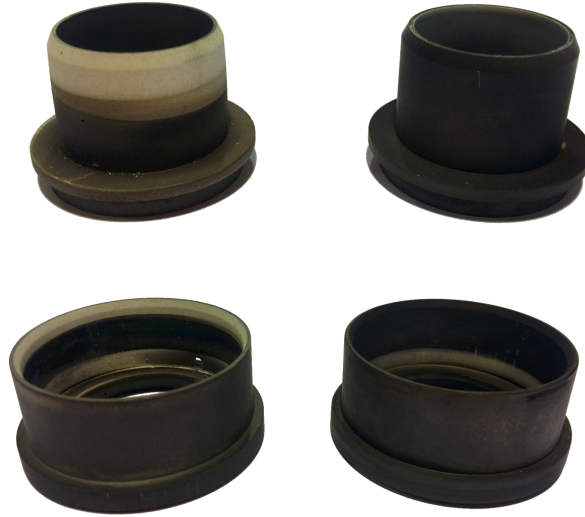
Figure 4.16: Ceramic walls of the ISCT200-US (left) and ISCT200-MS (right) highlighting, for the MS case, the absence of the characteristic erosion pattern in the black deposit formed on the walls.
