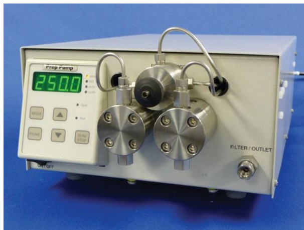
Figure 52: Pump used for water spray injection( Pre Pump SSI ).
