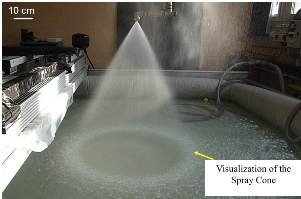
Figure 9: General Aspect of the Lecher nozzle employed in NPPin case of 3.5 bar and ambient temperature [10].
