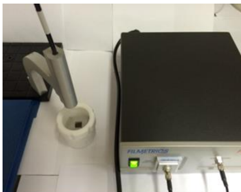
Figure 2-17. In situ measure of film thickness by visible reflectometry (VR).
