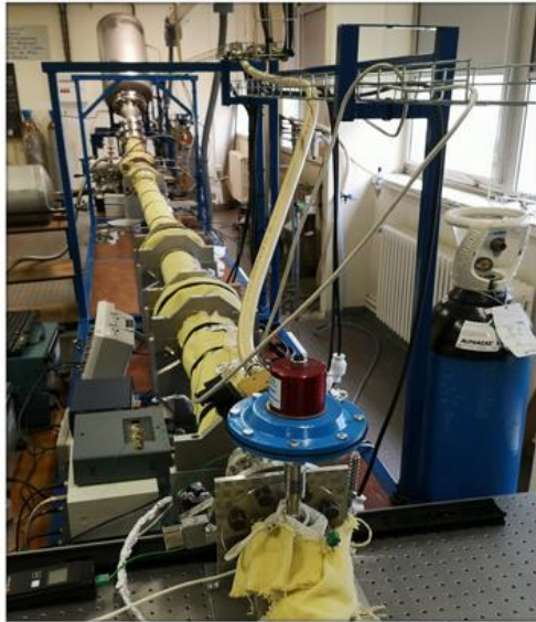
Figure 3.2: Real view of the heated shock tube, and a schematic diagram of the shock tube used in this work.
