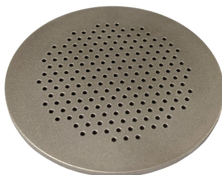
Figure 6.13: Photograph of the filter relative to the second prototype iodine tank.
