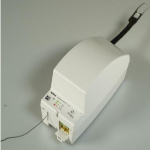
(a) We used iMet RS-41 radiosondes. These instruments measure temperatures from -90^{\circ}\text{C} to 50^{\circ}\text{C} with a resolution of 0.1^{\circ}\text{C} and an accuracy of 0.5^{\circ}\text{C} . Wind speed resolution is 0.1\text{ ms}^{-1} with an accuracy of 0.2\text{ ms}^{-1} .
