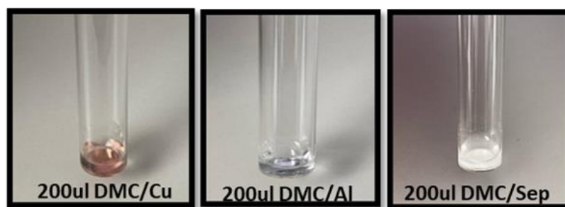
Figure 5-20 Non-electrochemically active battery components near 200 \mu\text{l} of DMC solvent inside 10mm NMR glass tube.
