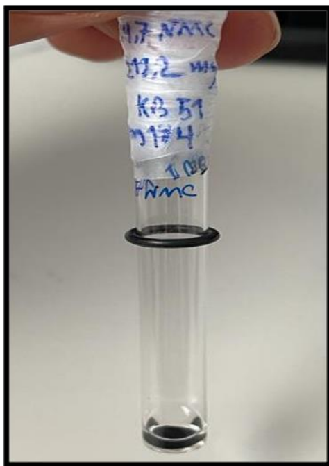
Figure 5-8 200 \mu l of liquid DMC solvent with 5mm pellet in 10 mm NMR glass tube wrapped with parafilm.
