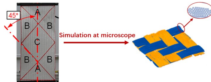
Figure 1.8 Modeling of reinforcements at the microscale: the fiber is treated as a homogeneous material.
