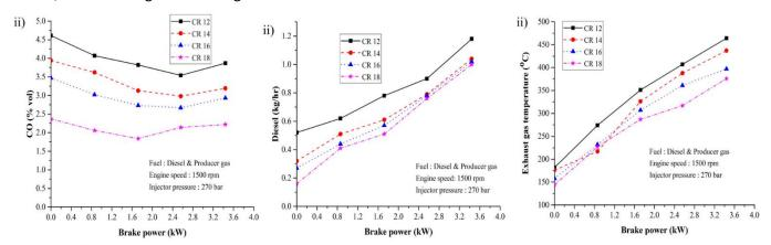
Figure 10: Results of Sharma and Kaushal [3] in dual-fuel producer gas/Diesel.
