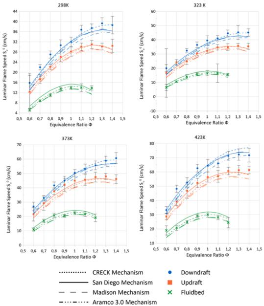
Figure 22: Experimental and simulated  $S_u^0$  results at 1 bar for four initial temperatures (298, 323, 373 and 423 K).
