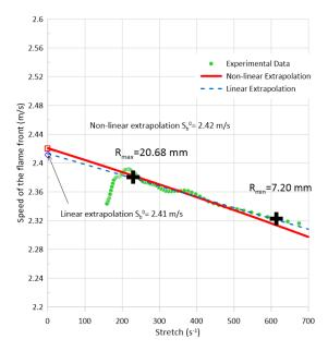
Figure 17: Example of flame speed evolution as a function of stretch - downdraft composition at 1 bar, 373 K and  $\phi = 1.2$ .
