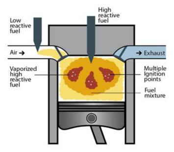
Figure 8: Illustration of the dual-fuel engine operation (image adapted from [186])
