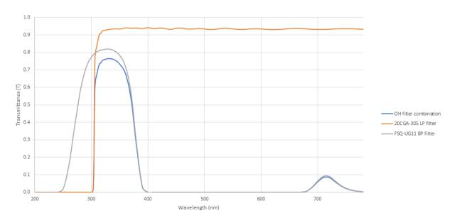
Figure 54: Filter combination used for OH\* chemiluminescence imaging.
