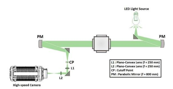
Figure 15: Schlieren Optical Set-up.
