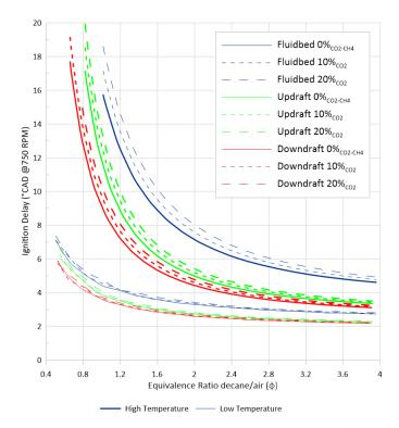
Figure 66: The effect of  $CO_2$  amount (from 0 to 20%) on the Ignition Delays of Syngas/Decane mixture for the 3 syngas compositions (Tin= 800K, Pin= 30 bar,  $\phi_{syngas/air}$  = 0.7 using the Madison Mechanism).
