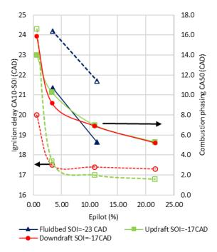
Figure 43: Effect of pilot fuel energy share on ignition delay (empty symbols, dashed lines) and combustion phasing CA50 (filled symbols, continuous lines) for three Syngas compositions (1200 RPM,  $P_{intake} = 1$  bar,  $T_{intake} = 300K$ ,  $\phi_{premixed} = 0.7$ ).
