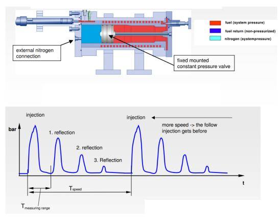
Figure 35: Schematic of the IAV injection analyzer used along with an example of the fuel of interest pressure trace (reproduced from the IAV Gmbh. brochure).
