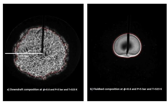
Figure 18: Example of the instabilities, thermal-diffusive (left) and buoyancy (right), we can obtain in this study.
