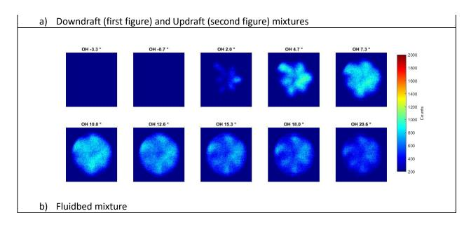
Figure 60: OH\* chemiluminescence images for the original compositions in a dual-fuel engine (a- Downdraft and Updraft and b- Fluidbed;  $\phi_{premixed}$ = 0.7, N= 750 RPM).
