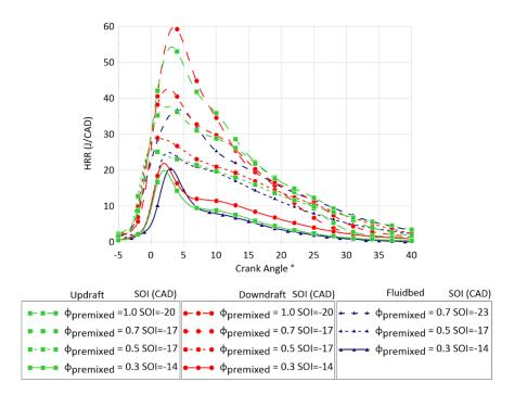
Figure 36: Evolution of Heat Release Rate for all premixed equivalence ratios and the three compositions (N=1200 RPM,  $P_{intake}$  = 1 bar,  $T_{intake}$  = 300K).
