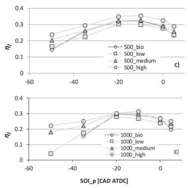
Figure 11: Fuel conversion efficiency ( $\eta_f$ ) of the dual-fuel, comparing the 3 ESS (35/50/65%:low/medium/high) and pilot fuel injection only (dashed line-'\_bio'), with two injection pressures, 500 and 1000 bar (adapted from the work of Carlucci et al. [90]).
