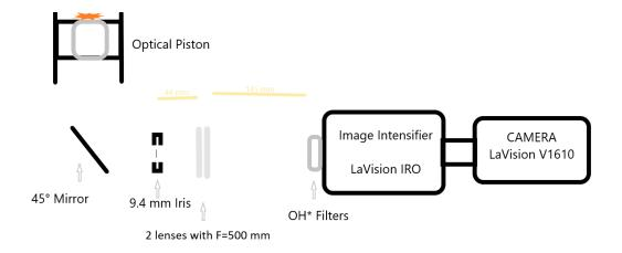
Figure 55: Optical imaging set-up for OH\* chemiluminescence.
