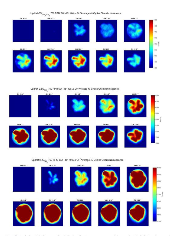
Figure 71: Effect of the CH4 share on the OH\* chemiluminescence averaged images for Updraft-based compositions ( $\phi_{syngas/air} = 0.7$ , N= 750 RPM).
