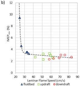
Figure 48: Relationship between a-combustion duration and b-stability (IMEP<sub>cov</sub>) as a function of syngas Laminar Flame Speed. (1200 RPM,  $P_{intake} = 1 \ bar$ ,  $T_{intake} = 300 \ K$ ,  $\phi_{premixed} = 0.7 \ SOI = -18 \ CAD \ BTDC$ )
