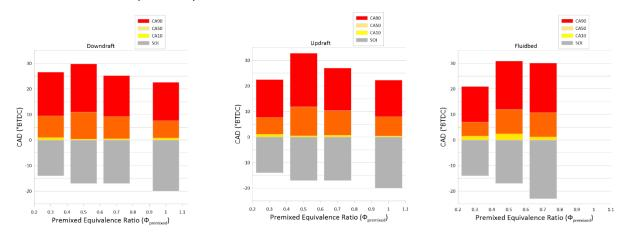
Figure 40: The effect of  $\phi_{premixed}$  on the combustion phasing (1200 RPM,  $P_{intake}$  = 1 bar,  $T_{intake}$  = 300K).
