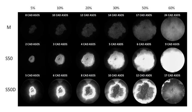
Figure 51: Example of natural luminosity of syngas stoichiometric flame for same flame area (5-10-20-30-50-60%) – M: methane, S50:  $50\%H_2$ -50%CO, S50D:  $25\%H_2$ -25%CO-15%CO<sub>2</sub>-35%N<sub>2</sub> (reprinted from Martinez-Boggio et al. [172]).
