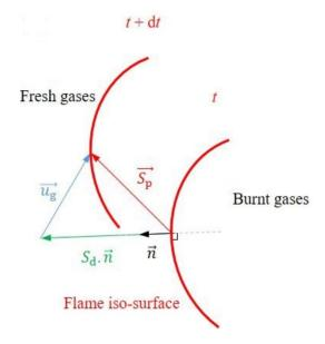
Figure 13: Schematic of the contours of local propagation and displacement speed of a premixed laminar flame (adapted from [96]).
