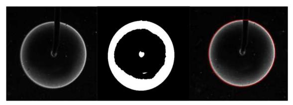
Figure 16: Post-processing steps illustrated by the unprocessed image (left), the binarized image (center) and the resulting flame contour traced over the unprocessed image (right).
