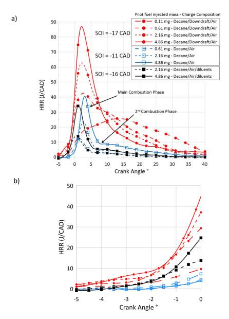
Figure 42: a- Heat release rate from the fuel pilot injection in air and air with diluents compared to Downdraft dual-fuel. ( $\phi_{premixed} = 0.7$ ) and b- zoom between -5 and 0 CAD.
