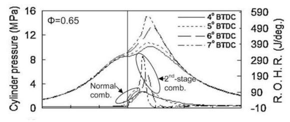
Figure 9: Example of a two Heat-Release Rate (HRR), reproduced from the work of Roy et al. [2].
