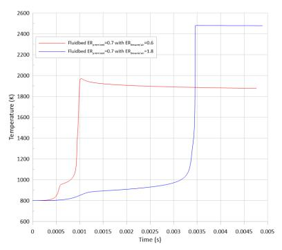
Figure 65: Temperature profiles of two  $\phi_{decane/air}$ , 0.6 and 1.8, mixed with a premixed charge of Fluidbed/air at  $\phi_{premixed}$ =0.7.
