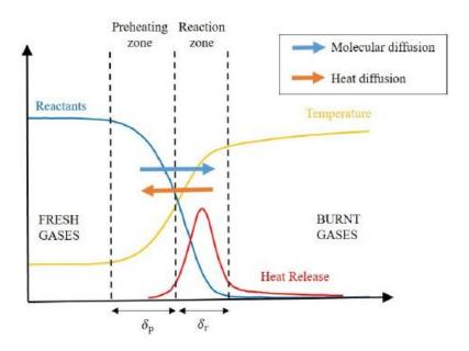
Figure 12: Schematic of a premixed flame (reproduced from [96]).
