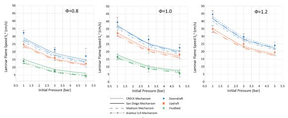
Figure 25: Comparison of the effect of pressure on the  $S_u^0$  for the three compositions at three equivalence ratios at  $T_{in}$ =323 K ( $\phi$ = 0.8, 1.0 and 1.2)
