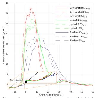
Figure 73: Effect of the CH<sub>4</sub> addition on the apparent Heat Release Rate (HRR) of dual-fuel operation of the compositions ( $\phi_{syngas/air}$  = 0.7, N= 750 RPM).
