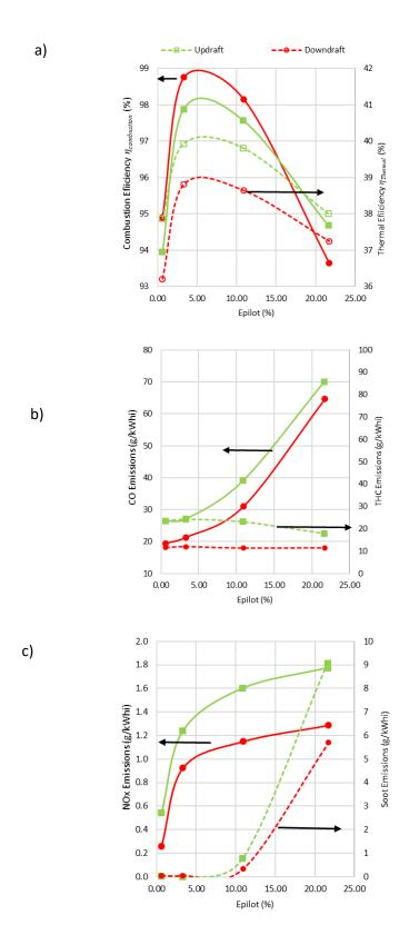
Figure 44: Efficiencies and emissions as a function of decane energy share for the three Syngas compositions. Filled symbols/continuous lines: a) Combustion efficiency, b) CO, c) NOx emissions. Empty symbols/Dashed lines: Thermal Efficiency, THC and Soot emissions for a, b and c respectively (1200 RPM,  $P_{intake} = 1 \ bar$ ,  $T_{intake} = 300 \ K$ ,  $\phi_{premixed} = 0.7$ ).
