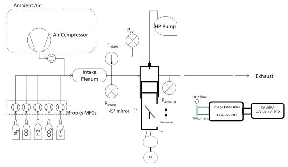
Figure 52: scheme of the optical engine set-up.
