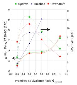
Figure 39: Effect of premixed equivalence ratio on ignition phasing (continuous lines) and first half of combustion (dotted lines) (N=1200 RPM Pintake = 1 bar Tintake = 300K).
