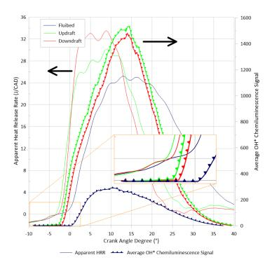
Figure 63: Comparison of the apparent Heat Release Ratio (HRR) and the OH\* chemilumunescence signals for the 3 original compositions ( $\phi_{premixed} = 0.7$ , N= 750 RPM).
