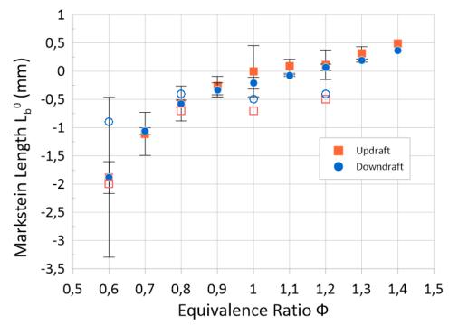
Figure 29: Zoom of the previous figure; experimental Markstein length results at 1 bar 298 K (filled symbols) compared to Monteiro et al. [5] results at 1 bar 293 K (empty symbols).
