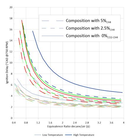
Figure 67: Effect of CH<sub>4</sub> variation in the reactive species in syngas on the IDT.
