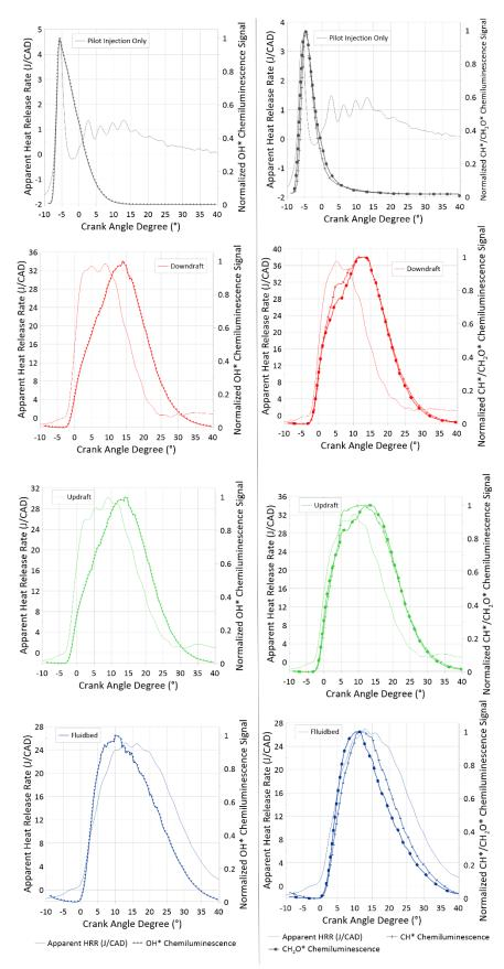
Figure 64: Comparison of the average apparent HRR with the normalized chemiluminescence of OH\* (left) and CH\*/CH<sub>2</sub>O\* (right) ( $\phi_{premixed}$  = 0.7, N= 750 RPM).
