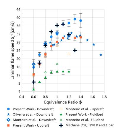
Figure 21: Comparison of  $S_u^0$  results at 1 bar 298 K with results from Monteiro et al. [5] (1 bar 293 K) and Oliveira et al. [7] (0.954 bar 298 K); methane  $S_u^0$  results provided by [133].
