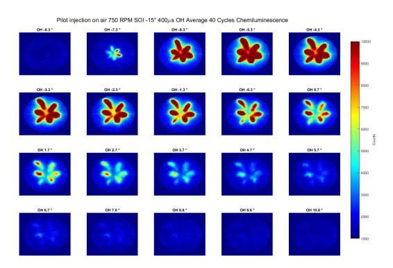
Figure 58: OH\* chemiluminescence images averaged on 40 cycles and the bar plot of the corresponding average signal for the pilot decane injection on air (without syngas, N=750 RPM).
