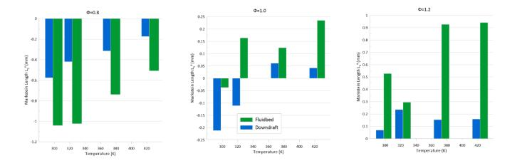
Figure 28: Markstein length results of the Fluidbed and the Downdraft compositions, for different temperatures and 3 equivalence ratios.
