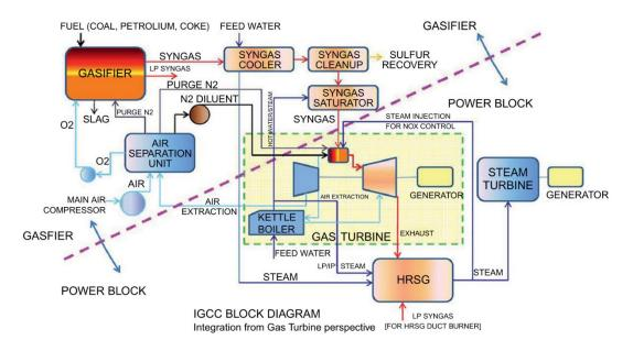
Figure 6: Diagram of IGCC (adapted from Ganjikunta [67])
