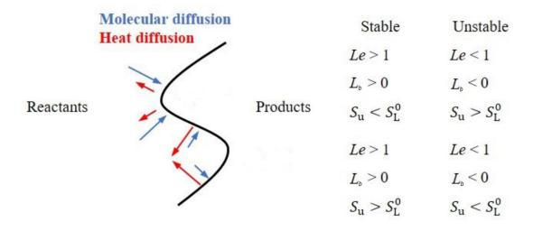
Figure 14: Relation of the Lewis number (Le) and the Markstein length ( $L_u$ , related to the burned  $L_b$  by the expansion ratio) with the flame stability (adapted from [96]).
