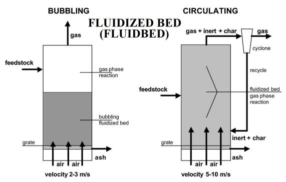
Figure 4: Common types of fixed and fluidized bed autothermal gasifiers (adapted from V. Belgiorno et al. [59]).
