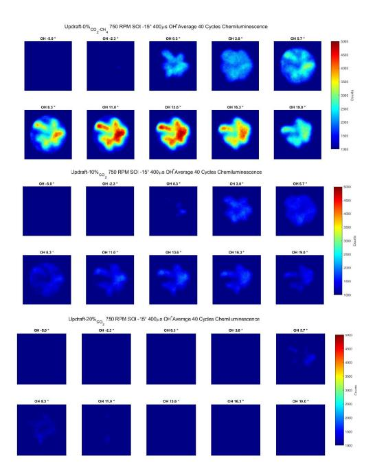
Figure 68: Effect of the  $CO_2$  share on  $OH^*$  chemiluminescence averaged images for Updraft-based compositions, ignited by the pilot injection ( $\phi_{syngas/air} = 0.7$ , N=750 RPM).
