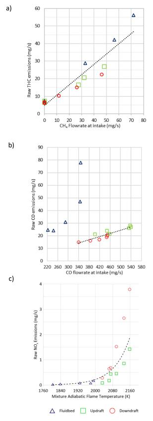
Figure 49: Relationship between THC emissions and intake CH<sub>4</sub> (a), Exhaust and Intake CO (b), NOx and  $T_{ad}$  (c) (1200 RPM,  $P_{intake} = 1 \ bar$ ,  $T_{intake} = 300 \ K$ ,  $\phi_{premixed} = 0.7 \ SOI = -18 \ CAD \ BTDC$ ).
