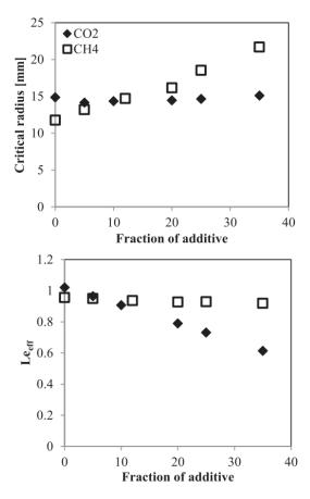
Figure 30: Effect of the addition of  $CO_2$  and  $CH_4$  on the effective Lewis number (Le<sub>eff</sub>) and the critical radius of the appearance of flame instabilities (adapted from Lapalme et al [128])
