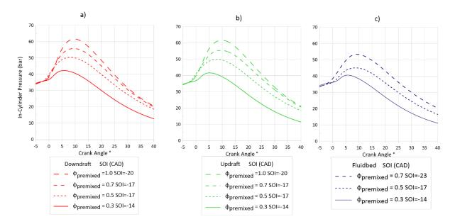
Figure 37. Evolution of In-Cylinder Pressure for all premixed equivalence ratio. (N=1200 RPM, P<sub>intake</sub> = 1 bar, T<sub>intake</sub> = 300K).
