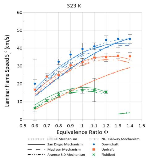
Figure 19: Example of experimental and simulated  $S_u^0$  results for 3 syngas compositions at 1 bar and 323 K.
