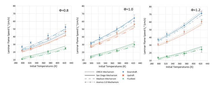
Figure 23: Kinetics mechanisms performances with varying the initial temperatures at three equivalence ratios.
