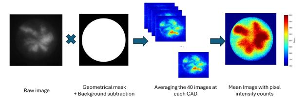
Figure 57: Schematic view of chemiluminescence image post-processing.
