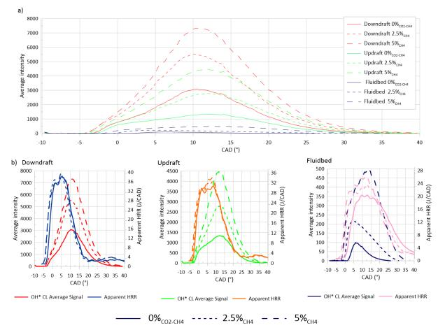
Figure 72: a- Effect of CH<sub>4</sub> on the average OH\* chemiluminescence signal b- Comparison of the OH\* average signal with the apparent Heat-Release Rate (HRR), grouped by the original composition ( $\phi_{syngas/air} = 0.7$ , N= 750 RPM).
