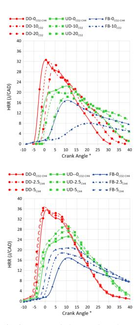
Figure 46: Heat Release Rate profiles for varying CO<sub>2</sub> (top) and CH<sub>4</sub> (bottom) contents (1200 RPM  $P_{intake} = 1 \, bar$ ,  $T_{intake} = 300 K$ ,  $\phi_{premixed} = 0.7 \, SOI = -18 \, CAD \, BTDC$ )
