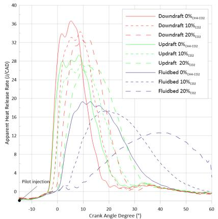
Figure 70: Effect of  $CO_2$  addition in total amount of dilution ( $N_2+CO_2$ ) on Heat Release Rate (HRR) for the 3 original compositions ( $\phi_{syngas/air} = 0.7$ , N=750 RPM).
