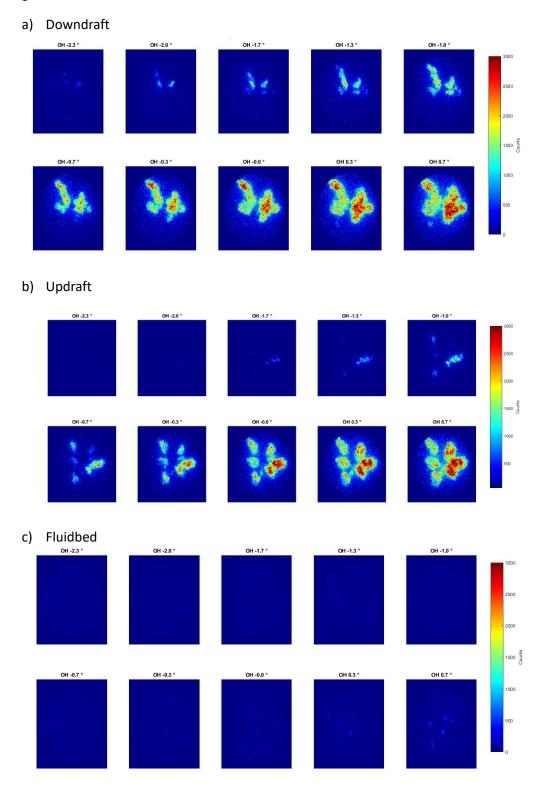
Figure 62: Instantaneous OH\* Image along same combustion cycle for the 3 original compositions ( $\phi_{premixed}$ = 0.7, N= 750 RPM).
