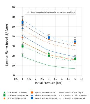
Figure 33: Effect of pressure and the decane addition for a fixed equivalence ratio ( $\phi_{syngas/air} = 0.7$ ) on the laminar flame speed ( $S_u^0$ ) (MF  $\rightarrow$  Mass Fraction).
