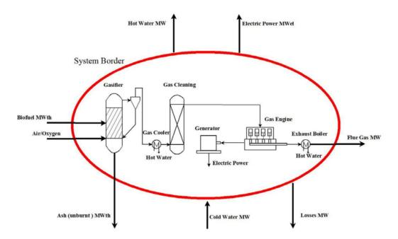
Figure 7: Schematic of a Combined Heat and Power (CHP) plant that uses an Internal Combustion Engine (ICE) (adapted from Brandin et al. [64])
