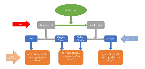
Figure 5: Product characteristics of allothermal and autothermal biomass gasification (adapted from R. Thomson et al. [50]).
