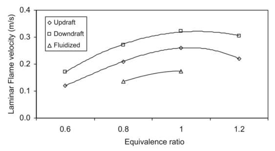
Figure 20: Unstretched laminar flame speed ( $S_u^0$ ) versus equivalence ratio ( $\phi$ ) plot of the 3 reference compositions at 293 K and 1 bar ((reproduced from the work of Monteiro et al. [5])
