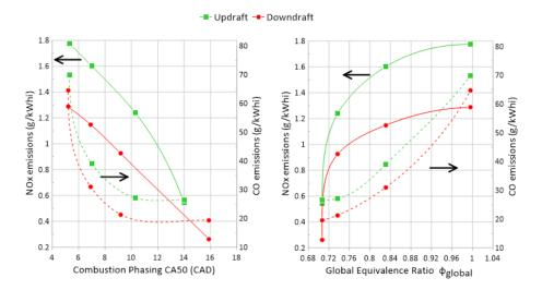
Figure 45: Specific emissions of NOx (continuous line) and CO (dashed line) as a function of combustion phasing (left) and global equivalence ratio (right) (1200 RPM  $P_{intake} = 1$  bar,  $T_{intake} = 300$ K,  $\phi_{premixed} = 0.7$ ).
