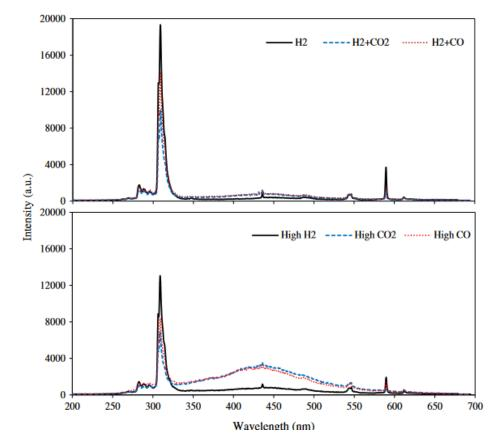
Figure 50: Example of chemiluminescence spectrum in syngas flame as a function of  $H_2$ , CO and  $CO_2$  concentration (reproduced from Huang et al. [162])
