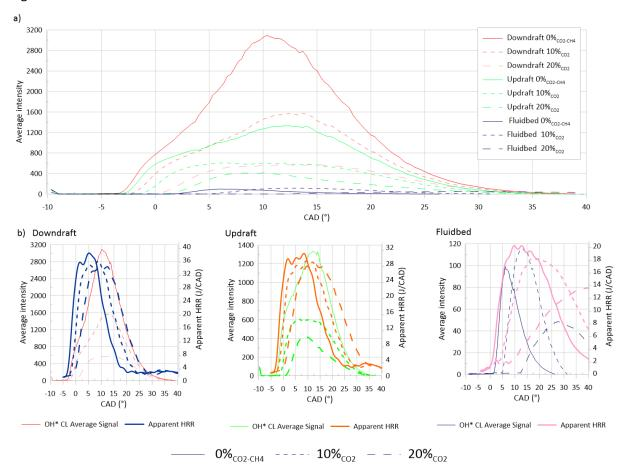
Figure 69: a- Effect of  $CO_2$  on the average OH\* chemiluminescence signal b- Comparison of the OH\* average signal with the apparent Heat-Release Rate (HRR), grouped by the original composition ( $\phi_{syngas/air} = 0.7$ , N= 750 RPM).
