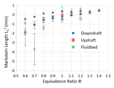
Figure 27: Present work experimental Markstein length results at 1 bar 298 K (filled symbols) compared to Monteiro et al. [5] results at 1 bar 293 K (empty symbols). Diamonds - Hydrogen at 1 bar and 298 K from [133].
