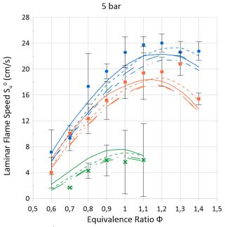
Figure 24: Experimental and simulated  $S_u^0$  results at 323 K initial temperature for 3 and 5 bar.
