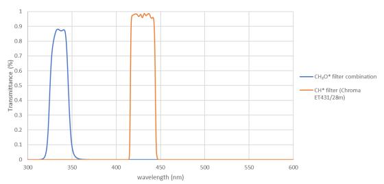
Figure 56: Filters used for the CH\* and CH₂O\* chemiluminescence
