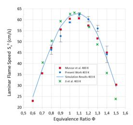
Figure 31:  $S_u^0$  of pure decane of the present work compared with simulation results [119] and literature data [139,140].
