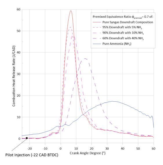
Figure 74: Example of Heat-Release Rate of Downdraft syngas as a function of ammonia shared quantity, ignition by decane pilot injection.
