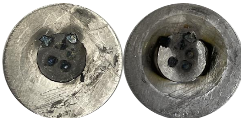
Figure 5.5 : Representative image of a 7.9 mm \phi , 270 \mu\text{m} thick, 106 mg holmium disc spot-welded to tantalum, before and after 68 minutes, 40 \mu\text{A} \cdot \text{h} PETtrace irradiation.
