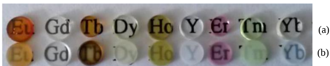
Figure 1.9.: Photography of polycrystalline glasses (a) and ceramics (b) diam. 5 mm, 1 mm thickness) obtained at CEMHTI laboratory by complete crystallization of the SrREGa 3 O 7 glass using a simple heat treatment. The samples are polished on 2 parallel faces 52 .
