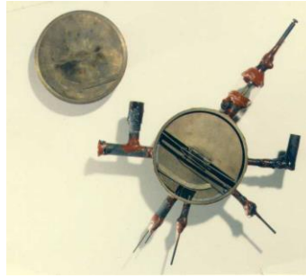
Figure 1.4: Lawrence's original cyclotron
