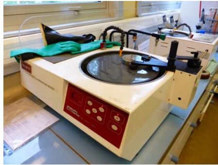
Figure 2.10: Polishing instrument (ESC 200 GTL (ESCIL company))
