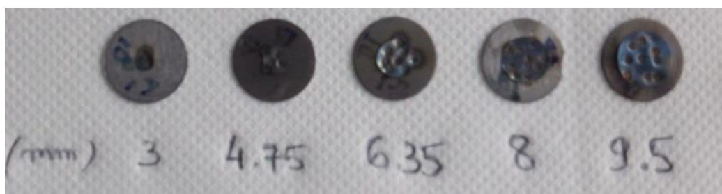
Figure 5.7: Determination of spot-beam by irradiation of 5 spot-welded targets with various diameter
