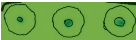
Figure 5.4: GAFchrom film of target 3.2 , 4.8 , and 6.5 \text{ mm} diameter irradiated on CTI-RDS-112
