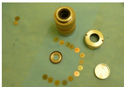
Figure 3.12: Stacked-foil sandwich for irradiation at 60°
