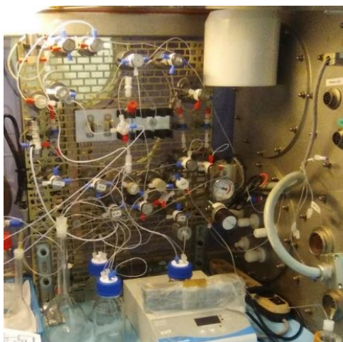
Figure 2.15: Set-up for automatization of ^{52}\text{Mn} production
