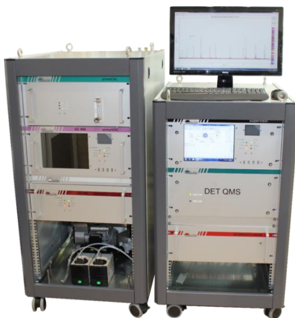
Figure II-1: Photo de la baie auto-TD-GC(C2C16)-FID/MS
