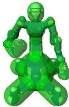
Figure 4.4: Self-collision avoidance model of DLR's humanoid Justin consisting of 28 convex hulls (left arm: 8, right arm: 8, mobile platform: 5, torso: 4, head: 2, floor: 1) (Dietrich, Wimbock, Taubig, et al., 2011)
