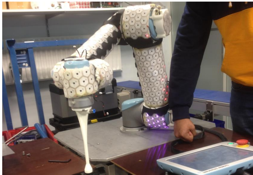
Figure 4.3: UR5 setup with the Artificial Robot Skin (Bharatheesha et al., 2017) showing some cells being activated (with red LEDs) by obstacles ( \leq 6 cm)
