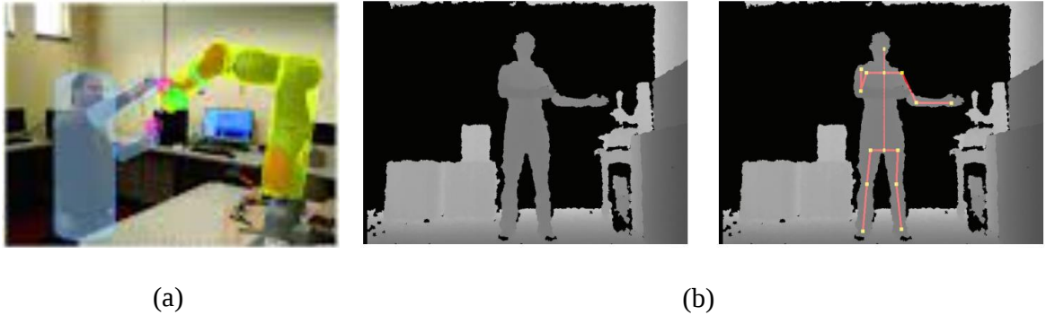
Figure 4.7: (a) The human is trying to touch the robot causing the robot to maneuver in a collision avoidance motion (Safeea, Neto, & Béarée, 2019) (b) Human body pose recognition from a single-view depth camera (Huang & Jeng, 2012)
