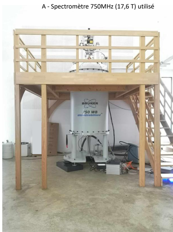
Figure 2-16 Description du montage de RMN in situ [121].
