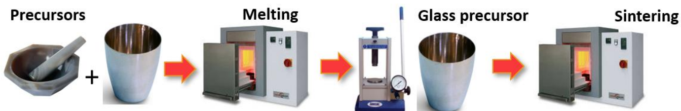
Fig. 4.1. Schematic of the glass crystallisation approach utilised in this work.
