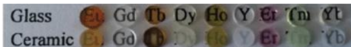
Fig. 1.10. The range of small RE melilite samples, SrREGa 3 O 7 (RE = Eu-Yb, Y), which could only be synthesised by a GC approach. The transparency observed in each sample is shown.
