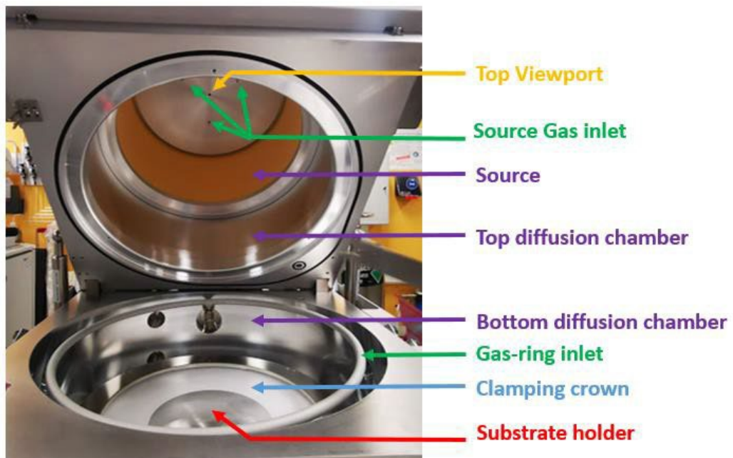
Figure II. 3: Schematized picture of the open Oxford Cobra ICP reactor chamber
