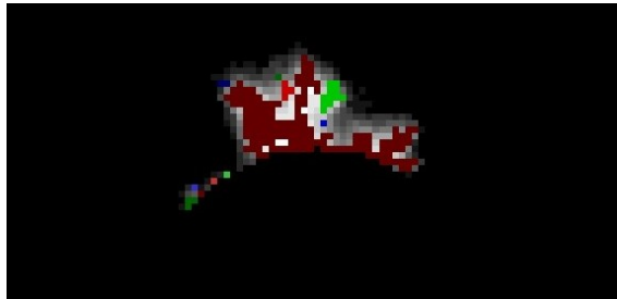
Figure 5.10: Largest spot cluster detected by the DFS algorithm, highlighted in brown. Picture taken 6.6 μs after discharge ignition.
